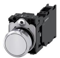
Pushbutton, 22 mm, round, metal, shiny, white, pushbutton, flat, momentary contact type, with holder, 1 NO+1 NC, spring-type terminal, with laser labeling, upper case and lower case, always upper case at the beginning of the word
