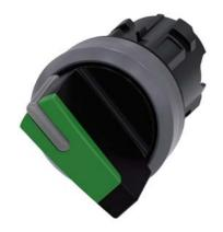
Selector switch, illuminable, 22 mm, round, plastic with metal front ring, green, selector switch, short, 2 switch positions O<I, momentary contact type, Actuating angle 45°, 10:30h/12h, Z=50-unit packaging
