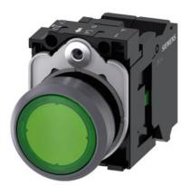
Illuminated pushbutton, 22 mm, round, plastic with metal front ring, green, pushbutton, flat, momentary contact type, with holder, 1NO, LED module with integrated LED 24 V AC/DC, spring-type terminal, with laser labeling, inscription or symbol Customer-specific selection with SIRIUS ACT configurator (CIN)
