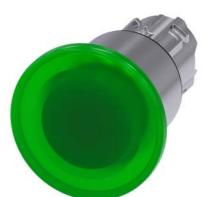
Illuminated mushroom pushbutton, 22 mm, round, metal, shiny, green, 40 mm, 3 switch positions, latches after pushing in, unlatches by pull-tounlatch mechanism to center position, after pulling out the button Retraction to center position, with laser labeling, upper case
