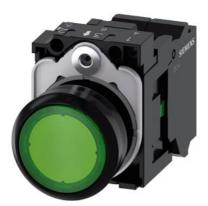
Illuminated pushbutton, 22 mm, round, plastic, green, pushbutton, flat, momentary contact type, with holder, 1NO, LED module with integrated LED 24 V AC/DC, spring-type terminal, with laser labeling, inscription or symbol Customer-specific selection with SIRIUS ACT configurator (CIN)
