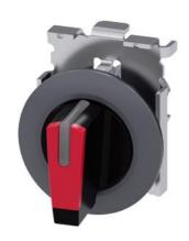
Selector switch, illuminable, 30 mm, round, Metal, matte, red, selector switch, short, front ring for flush installation, 3 switch positions I-O-II, latching, actuating angle 2x45°, 10:30h/12h/13:30h, Z=50-unit packaging
