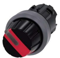
Selector switch, illuminable, 22 mm, round, plastic with metal front ring, red, Rotary knob, 2 switch positions O-I, latching, actuating angle 90°, 10:30h/13:30h, with laser labeling, inscription or symbol Customer-specific selection with SIRIUS ACT configurator (CIN)
