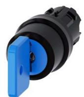
Key-operated switch O.M.R, 22 mm, round, plastic, lock number 73038, blue, with 2 keys, 3 switch positions I-O-II, latching, actuating angle 2x45°, 10:30h/12h/13:30h, Key removal I+O+II, with laser labeling, lower case
