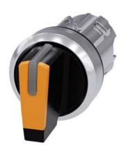
Selector switch, illuminable, 22 mm, round, metal, shiny, amber, selector switch, short, 3 switch positions I>O<II, momentary contact type, actuating angle  $2x45^{\circ}$ , 10:30h/12h/13:30h, Z=50-unit packaging
