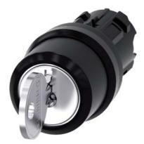
RONIS key-operated switch, 22 mm, round, plastic, lock number SB30, with 2 keys, 3 switch positions I-O-II, latching, actuating angle 2x45°, 10:30h/12h/13:30h, Key removal I+II, possible special locks: SB31, 421, 455, with laser labeling, lower case
