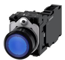
Illuminated pushbutton, 22 mm, round, plastic, blue, pushbutton, flat, momentary contact type, with holder, 1 NO+1 NC, LED module with integrated LED 110 V AC, screw terminal, with laser labeling, symbol number according to, ISO 7000 or IEC 60417
