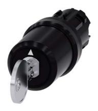
Key-operated switch BKS, 22 mm, round, plastic, lock number S1, with 2 keys, 3 switch positions I-O<II, left latching, right momentary contact type, actuating angle 2x45°, 10:30h/12h/13:30h, key removal I, with laser labeling, upper case and lower case, always upper case at beginning of line
