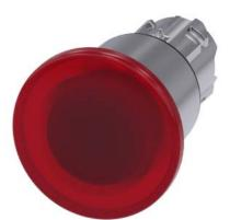
Illuminated mushroom pushbutton, 22 mm, round, metal, shiny, red, 40 mm, 3 switch positions, latches after pushing in, unlatches by pull-tounlatch mechanism to center position, after pulling out the button Retraction to center position, with laser labeling, symbol number according to, ISO 7000 or IEC 60417
