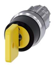
Key-operated switch O.M.R, 22 mm, round, metal, shiny, lock number 73033, yellow, with 2 keys, 3 switch positions I>O<II, momentary contact on the left, latching on the right, actuating angle 2x45°, 10:30h/12h/13:30h, Key removal II, with laser labeling, upper case and lower case, always upper case at beginning of line
