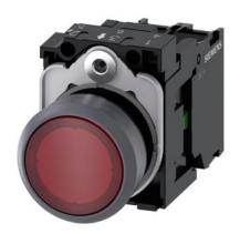
Illuminated pushbutton, 22 mm, round, plastic with metal front ring, red, pushbutton, flat, momentary contact type, with holder, 1NO, LED module with integrated LED 24 V AC/DC, screw terminal, Z=20-unit packaging
