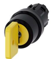
Key-operated switch O.M.R, 22 mm, round, plastic, lock number 73033, yellow, with 2 keys, 3 switch positions I-O-II, latching, actuating angle 2x45°, 10:30h/12h/13:30h, Key removal I+O+II, with laser labeling, upper case and lower case, always upper case at the beginning of the word
