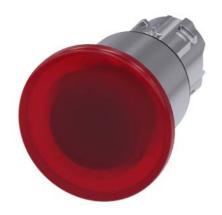
Illuminated mushroom pushbutton, 22 mm, round, metal, shiny, red, 40 mm, 3 switch positions, latches after pushing in, unlatches by pull-to-unlatch mechanism to center position, after pulling out the button Retraction to center position, Z=50-unit packaging
