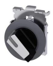
Selector switch, illuminable, 30 mm, round, Metal, matte, white, selector switch, short, front ring for flush installation, 2 switch positions O-I, latching, actuating angle 90°, 10:30h/13:30h, with laser labeling, inscription or symbol Customer-specific selection with SIRIUS ACT configurator (CIN)
