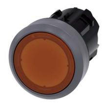
Illuminated pushbutton, 22 mm, round, plastic with metal front ring, amber, pushbutton, flat momentary contact type, Z=100-unit packaging
