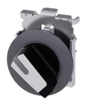
Selector switch, illuminable, 30 mm, round, Metal, matte, white, selector switch, short, front ring for flush installation, 2 switch positions O<I, momentary contact type, Actuating angle 45°, 10:30h/12h, with laser labeling, inscription or symbol Customer-specific selection with SIRIUS ACT configurator (CIN)
