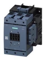
power contactor, AC-3 185 A, 90 kW / 400 V AC (50-60 Hz) / DC operation 23-26 V AC/DC (spring-loaded terminal auxiliary contacts 2 NO + 2 NC 3-pole, frame size S6E busbar connections drive: conventional with 2 box terminals 3RT19 55-4G up to 70 mm
