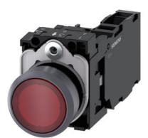
Illuminated pushbutton, 22 mm, round, plastic with metal front ring, red, pushbutton, flat, momentary contact type, with holder, 1 NO+1 NC, LED module with integrated LED 110 V AC, screw terminal, with laser labeling, upper case and lower case, always upper case at beginning of line
