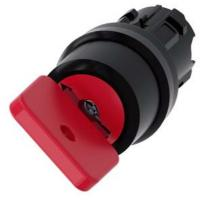
Key-operated switch O.M.R, 22 mm, round, plastic, lock number 73037, red, with 2 keys, 2 switch positions O-I, latching, actuating angle 90°, 10:30h/13:30h, key removal O+I, with laser labeling, upper case
