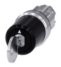
key-operated switch Siemens, 22 mm, round, metal, shiny, special lock, with 2 keys, 3 switch positions I-O-II, latching, actuating angle 2x45°, 10:30h/12h/13:30h, key removal I+O+II
