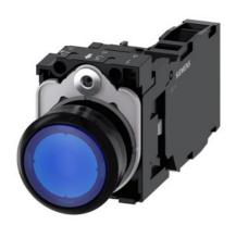
Illuminated pushbutton, 22 mm, round, plastic, blue, pushbutton, flat, momentary contact type, with holder, 1 NO+1 NC, LED module with integrated LED 24 V AC/DC, screw terminal, with laser labeling, inscription or symbol Customer-specific selection with SIRIUS ACT configurator (CIN)
