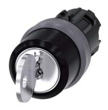
RONIS key-operated switch, 22 mm, round, plastic with metal front ring, lock number SB30, with 2 keys, 3 switch positions I-O-II, latching, actuating angle 2x45°, 10:30h/12h/13:30h, Key removal II, possible special locks: SB31, 421, 455, with laser labeling, lower case
