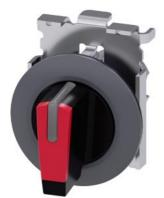
Selector switch, illuminable, 30 mm, round, Metal, matte, red, selector switch, short, front ring for flush installation, 3 switch positions I-O-II, latching, actuating angle  $2x45^{\circ}$ , 10:30h/12h/13:30h, with laser labeling, upper case
