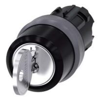
RONIS key-operated switch, 22 mm, round, plastic with metal front ring, special lock, with 2 keys, 3 switch positions I-O<II, left latching, right momentary contact type, actuating angle 2x45°, 10:30h/12h/13:30h, key removal O+I, possible special locks: SB31, 421, 455
