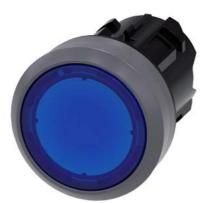
Illuminated pushbutton, 22 mm, round, plastic with metal front ring, blue, pushbutton, flat, latching, Push-to-release mechanism, with laser labeling, upper case and lower case, always upper case at beginning of line
