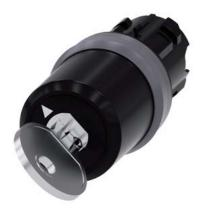
key-operated switch Siemens, 22 mm, round, plastic with metal front ring, lock no. LSG1, with 2 keys, 2 switch positions O<I, momentary contact type, actuating angle 45°, 10:30h/12h, key removal O, with laser labeling, upper case
