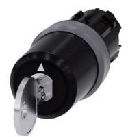
key-operated switch Siemens, 22 mm, round, plastic with metal front ring, special lock, with 2 keys, 3 switch positions I>O<II, momentary contact on the left, latching on the right, actuating angle 2x45°, 10:30h/12h/13:30h, key removal II
