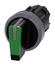
Selector switch, illuminable, 22 mm, round, plastic with metal front ring, green, selector switch, short, 3 switch positions I-O<II, left latching, right momentary contact type, actuating angle 2x45°, 10:30h/12h/13:30h, with laser labeling, inscription or symbol Customer-specific selection with SIRIUS ACT configurator (CIN)
