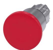
Mushroom pushbutton, 22 mm, round, metal, shiny, red, 40 mm, 3 switch positions, latches after pushing in, unlatches by pull-to-unlatch mechanism to center position, after pulling out the button Retraction to center position, with laser labeling, upper case
