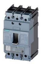
circuit breaker 3VA5 UL frame 125 breaking capacity class M 35kA @ 480 V 3-pole, line protection TM230, FTAM, In=35A overload protection Ir=35A fixed short-circuit protection li=5...10 x In cable connection on both sides
