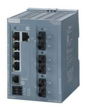
SCALANCE XB205-3 managed Layer 2 IE switch 5x 10/100 Mbit/s RJ45 ports 3x MM FO ST port 1x console port, diagnostics LED redundant power supply; IEC 62443-4-2 certified; temperature range 0 °C to +60 °C DIN-rail mounting; default EtherNet/IP.
