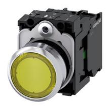
Illuminated pushbutton, 22 mm, round, metal, shiny, yellow, pushbutton, flat, momentary contact type, with holder, 1NO, LED module with integrated LED 24 V AC/DC, screw terminal, with laser labeling, lower case
