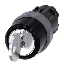
RONIS key-operated switch, 22 mm, round, plastic with metal front ring, lock number SB30, with 2 keys, 3 switch positions I-O-II, latching, actuating angle 2x45°, 10:30h/12h/13:30h, Key removal I+O+II, possible special locks: SB31, 421, 455 Z=50-unit packaging
