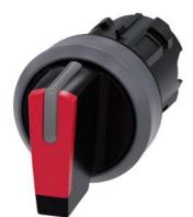
Selector switch, illuminable, 22 mm, round, plastic with metal front ring, red, selector switch, short, 3 switch positions I>O<II, momentary contact type, actuating angle  $2x45^{\circ}$ , 10:30h/12h/13:30h, with laser labeling, upper case and lower case, always upper case at the beginning of the word
