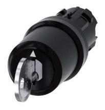
Key-operated switch IKON, 22 mm, round, plastic, lock number 360012K1, with 2 keys, 3 switch positions I-O<II, left latching, right momentary contact type, actuating angle 2x45°, 10:30h/12h/13:30h, key removal O+I, with laser labeling, upper case and lower case, always upper case at the beginning of the word
