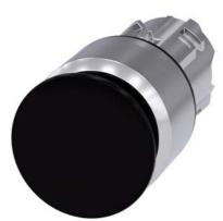
Mushroom pushbutton, 22 mm, round, metal, shiny, black, 30 mm, latching, pull-to-unlatch mechanism, with laser labeling, upper case and lower case, always upper case at the beginning of the word
