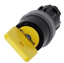
Key-operated switch O.M.R, 22 mm, round, plastic with metal front ring, lock number 73033, yellow, with 2 keys, 2 switch positions O-I, latching, actuating angle 90°, 10:30h/13:30h, key removal O+I, with laser labeling, upper case and lower case, always upper case at beginning of line
