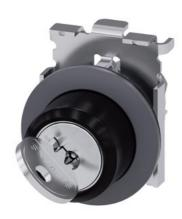
RONIS key-operated switch, 30 mm, round, Metal, matte, front ring for flush installation, special lock, with 2 keys, 2 switch positions O<I, momentary contact type, Actuating angle  $45^\circ,\,10:30h/12h,$  key removal O, possible special locks: SB31, 421, 455
