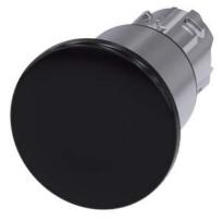
Mushroom pushbutton, 22 mm, round, metal, shiny, black, 40 mm, 3 switch positions, latches after pushing in, unlatches by pull-to-unlatch mechanism to center position, after pulling out the button Retraction to center position, Z=50-unit packaging
