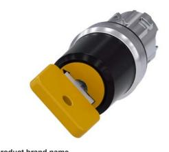
Key-operated switch O.M.R, 22 mm, round, metal, shiny, lock number 73033, yellow, with 2 keys, 2 switch positions O-I, latching, actuating angle 90°, 10:30h/13:30h, key removal O+I, with laser labeling, upper case and lower case, always upper case at beginning of line
