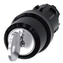
RONIS key-operated switch, 22 mm, round, plastic, lock number SB30, with 2 keys, 3 switch positions I-O-II, latching, actuating angle 2x45°, 10:30h/12h/13:30h, key removal O, possible special locks: SB31, 421, 455, with laser labeling, lower case
