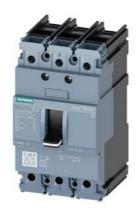
circuit breaker 3VA5 UL frame 125 breaking capacity class S 25kA @ 480 V 3-pole, line protection TM210, FTFM, In=20A overload protection Ir=20A fixed short-circuit protection Ii=15 x In UL489 SB (naval), 50 deg. cel. cable connection on both sides
