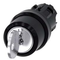
RONIS key-operated switch, 22 mm, round, plastic, lock number SB30, with 2 keys, 3 switch positions I-O<II, left latching, right momentary contact type, actuating angle 2x45°, 10:30h/12h/13:30h, key removal I, possible special locks: SB31, 421, 455, with laser labeling, inscription or symbol Customer-specific selection with SIRIUS ACT configurator (CIN)
