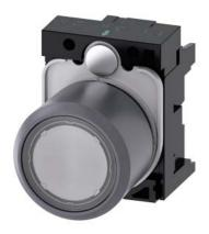
Pushbutton, compact, with extended stroke (12 mm), 22 mm, round, plastic with metal front ring, clear, pushbutton, flat, momentary contact type, with holder, with laser labeling, upper case and lower case, always upper case at beginning of line
