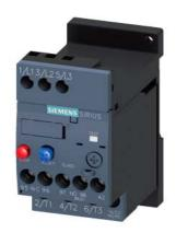
Overload relay 0.14...0.20 A Thermal For motor protection Size S00, Class 10 Stand-alone installation Main circuit: Screw Auxiliary circuit: Screw Manual-Automatic-Reset
