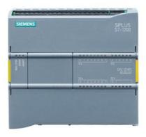
SIPLUS S7-1200 CPU 1214FC DC/DC/DC based on 6ES7214-1AF40-0XB0 with conformal coating, -25...+55  $^{\circ}$ C, compact CPU, DC/DC/DC, onboard I/O: 14 DI 24 V DC; 10 DQ 24 V DC; 2 AI 0-10 V DC, power supply: DC 20.4-28.8 V DC, program/data memory 125 KB
